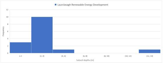
Plate 8-1: Histogram of subsoil depths across the Proposed Wind Farm Site (from borehole data)
